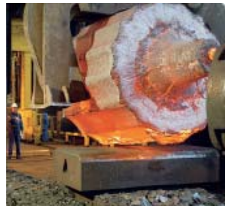
Depositing a heavy ingot on the 55 MN open-die forging press
