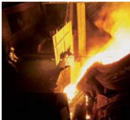
Tapping slag at the ladle furnace in the steel mill
