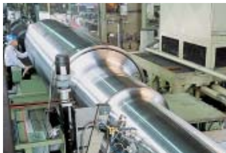
Automated ultrasonic testing of a generator shaft
