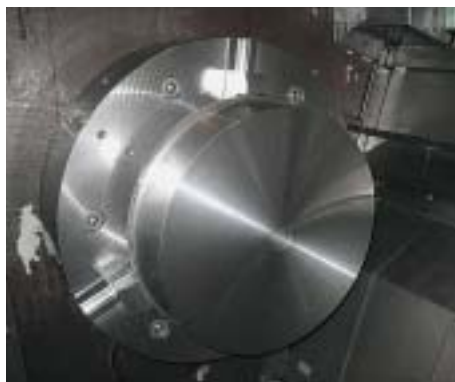
Gearwheel blank being machined
