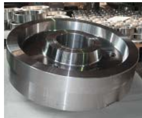
Gearwheel blank for a special marine transmission ready for dispatch
