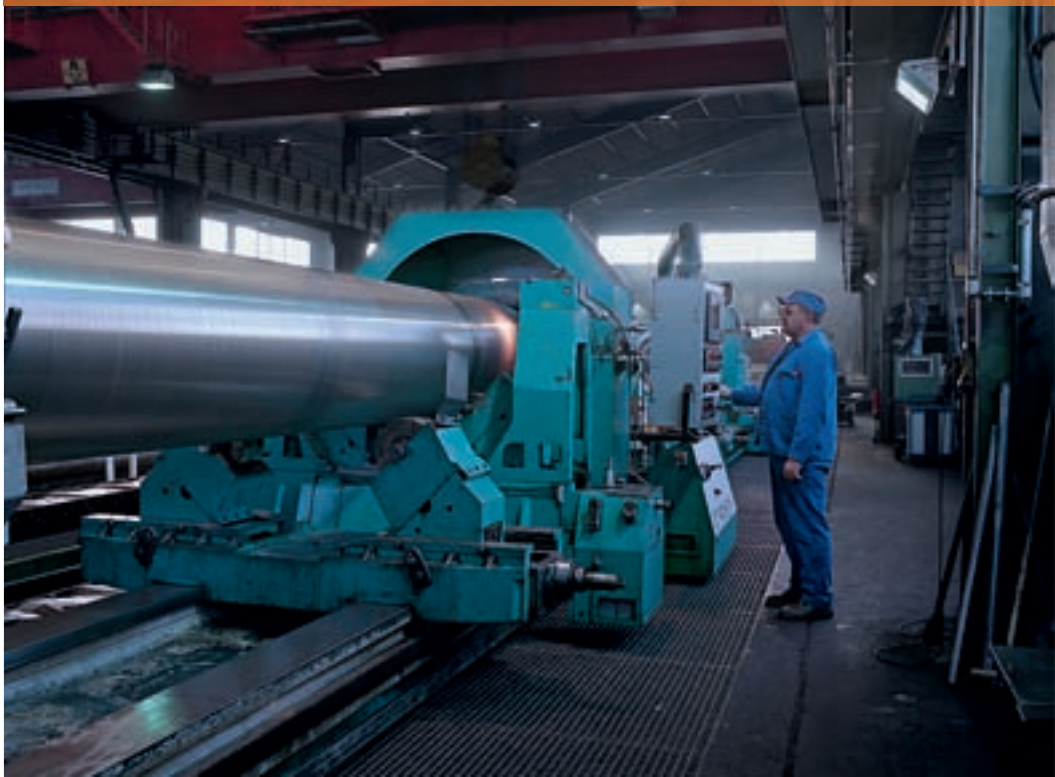
Harald Lackmann operates the horizontal boring machine during face milling
