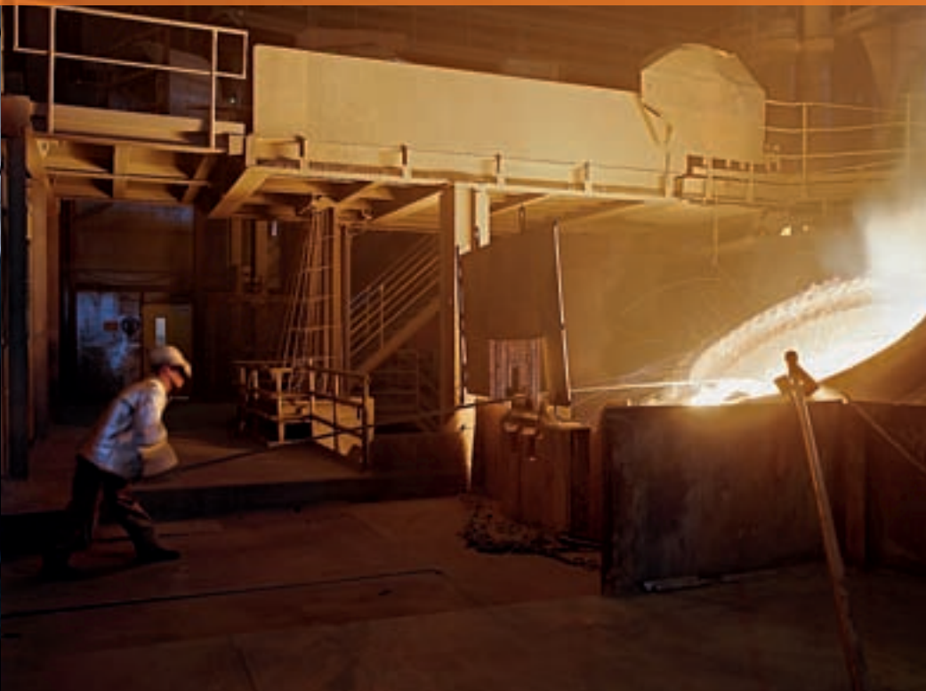
Removing slag during secondary metallurgy
