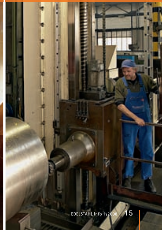
Jürgen Cross conducting an axial boring operation
