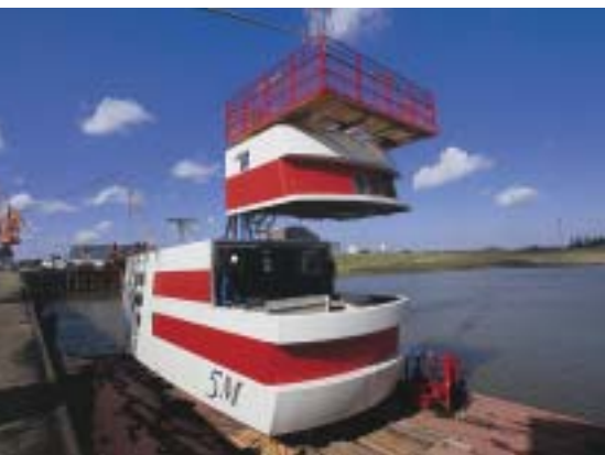
The machine housing comprising gear steel from Wetzlar is assembled on the ground – The complete power house is fitted in one piece – The complete 5M wind power generator (from left to right)
