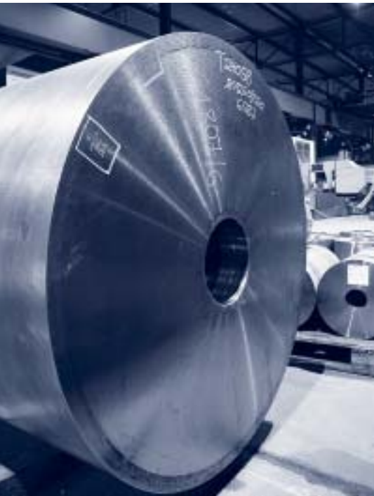
Structural steel is stocked for making gears up to 1,400 mm
