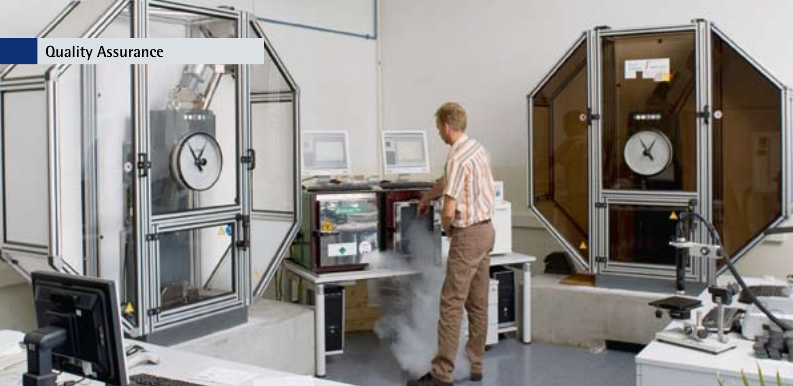
Impact testing equipment in the mechanical laboratory
