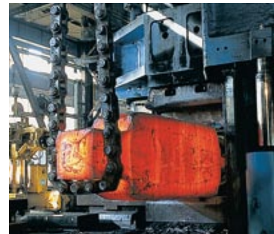
Heavy ingot on the 55 MN press
