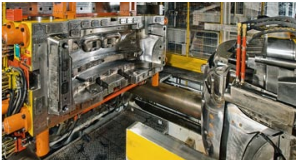
Core and mould side in the production cycle
