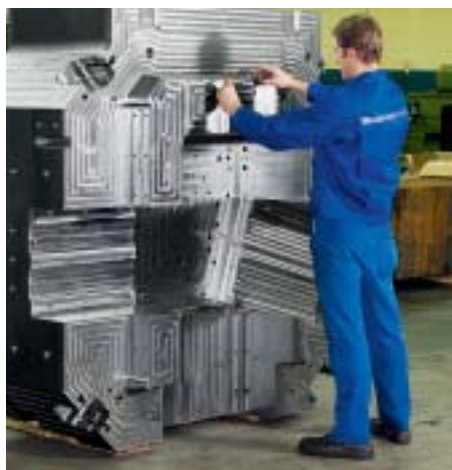
Dimensional check of a holding block
